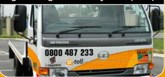
The LTRU is tasked with moving stranded or accident-damaged vehicles (predominantly passenger cars) out of the roadway. These units employ rollback-type towing trucks (i.e. having a flat loadbed onto which a car can be loaded) a place where it will not be in danger and obstruct the flow of traffic.
