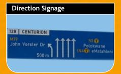
Blue direction signs are erected along dual carriageways to guide motorists in selecting an exit ramp close to a road
